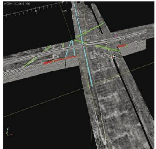
At Safedigging we use the very latest Electromagnetic Utility Detectors from the market leader Vivax-Metrotech, IDS Stream C GPR & Opera Duo. Using Gred HD Post Processing Software and One Vision we are able to completely Post Process the data collected so you have the confidence everything is covered, giving you the very best information possible sub surface.
